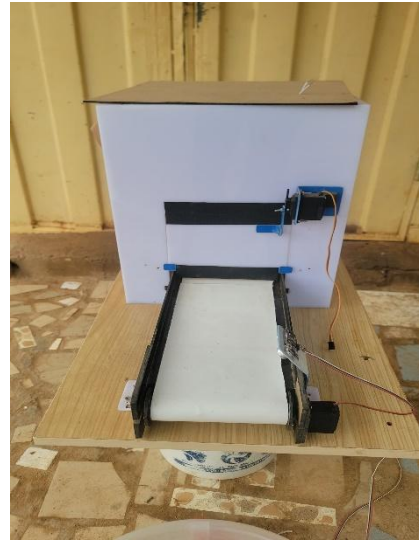
Plate 3.2 Conveyor Housing, Belt and Ultrasonic sensor
