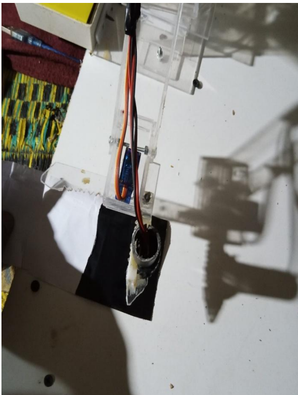
Fig. 10: Gripper opens at the picking point when it senses a black object.
