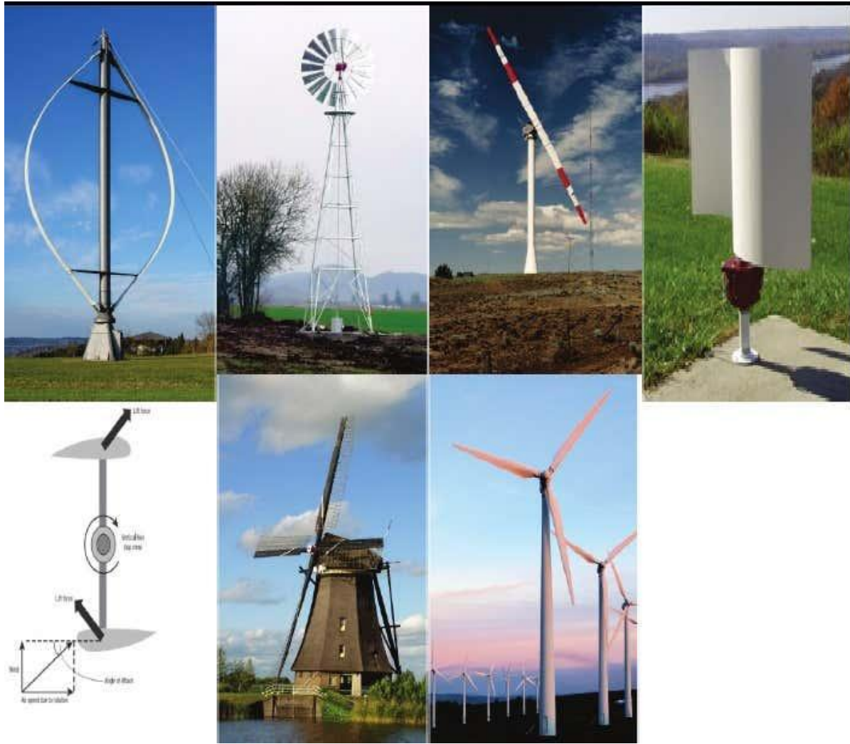
Fig. 2: Wind turbine designs: (a) Darrieus, (b) American water pumper, (c) 2-blade design, (d) Savonius, (e) Dutch 4-arms (g) 3-blade design.
