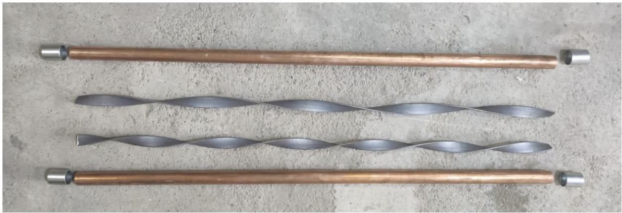
Figure (4) twisted tape and inner pipe
