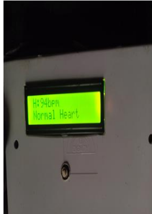
Fig. 12(a): The implemented system's reading indicates a normal heartbeat rate
