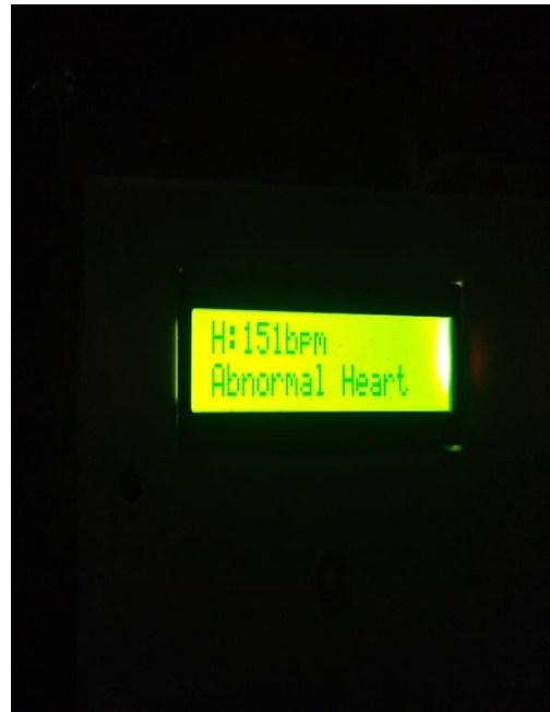
Fig. 13: The implemented system's reading indicates an irregular cardiac rate
