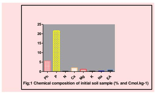
Fig. 1: Represents the chemical composition of the initial soil sample and their level of concentrations. According to the figure, the pH level of the initial soil sample is acidic in nature. Phosphorus was ranked highest in the level of concentration when compared with the other chemical compositions such as N, Ca, Mg, K, Na, and EA in the soil.
