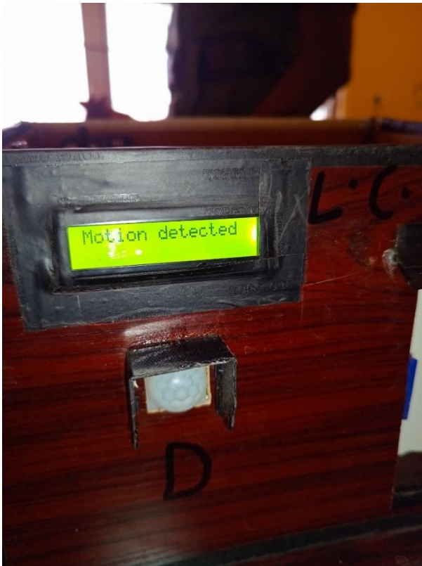
Figure 4.9(b): Motion detected with the help of PIR sensor used
