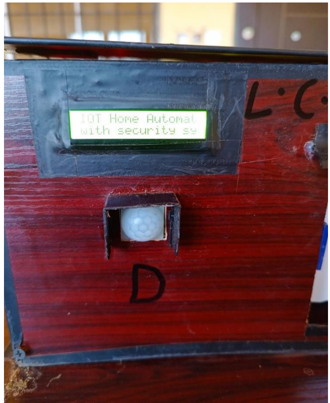
Figure 4.4: The Passive Infrared Sensor that is used to detect motion, if there is an intrusion labeled D.
