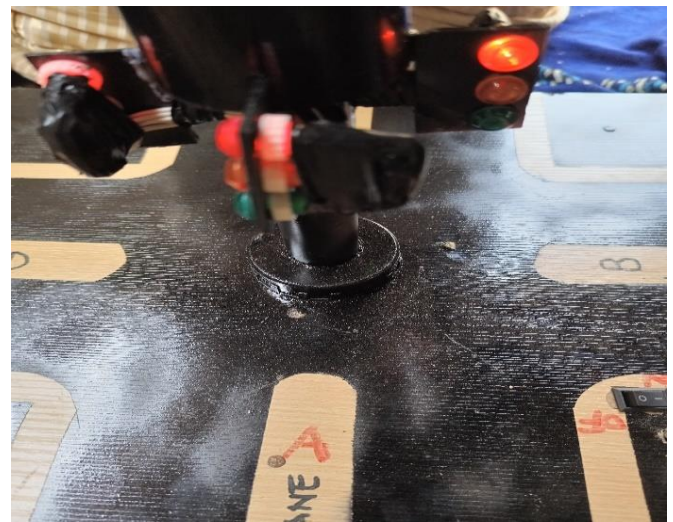
Fig. 8: Lane A is displaying red (L.E.D.), which is stop
