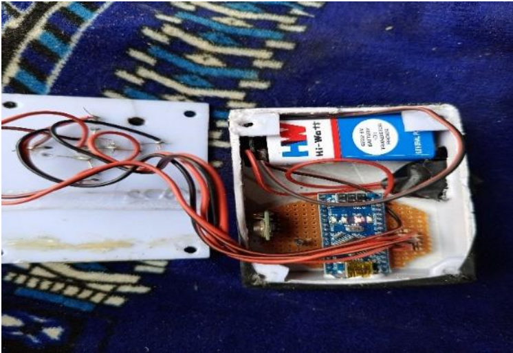
Fig. 1: The internal circuitry of the control switch.
