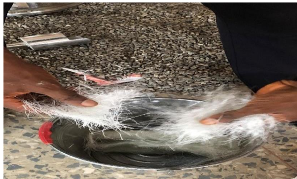
Fig. 4. Alkali resistant glass fiber matrix (chopped strands)
