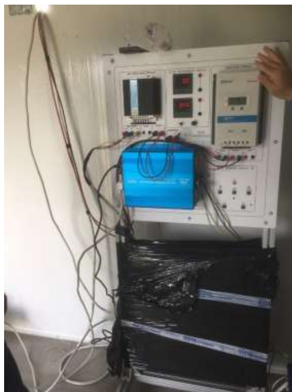
Figure-4: The complete compact control panel unit consisting of Solar Charge Controller, Wind Turbine Charge Controller, AC/DC Measurement Module, PC Interface Module, DC/AC Inverter.
