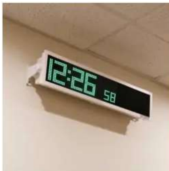
Figure 2: Modern Wireless LED Message Board: For Text Messaging and Digital Time Display
