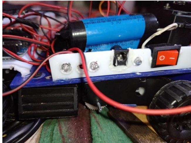
Figure 7: The three LEDs that are used in the system
