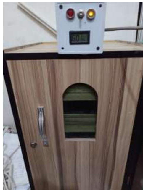
Fig. 2. The construction of the whole egg incubator
