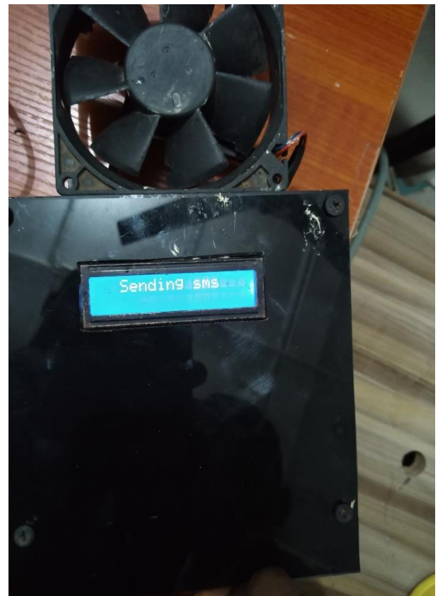
Fig. 6: The system sends an SMS to the registered mobile number
