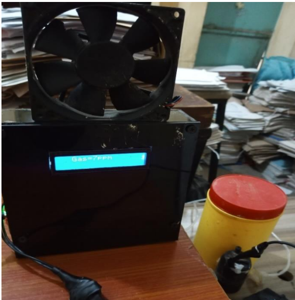
Fig. 4: Gas leakage was not detected as a result of the implementation
