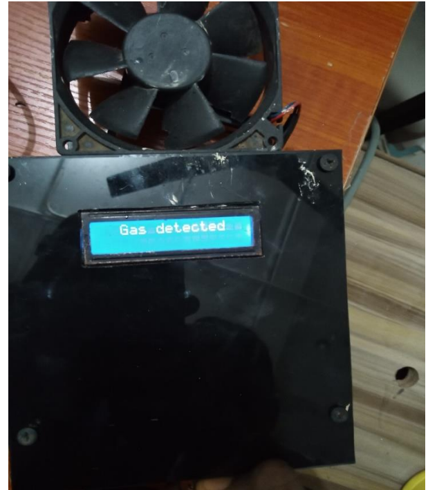
Fig. 5: The implementation result shows there is LPG present in the environment
