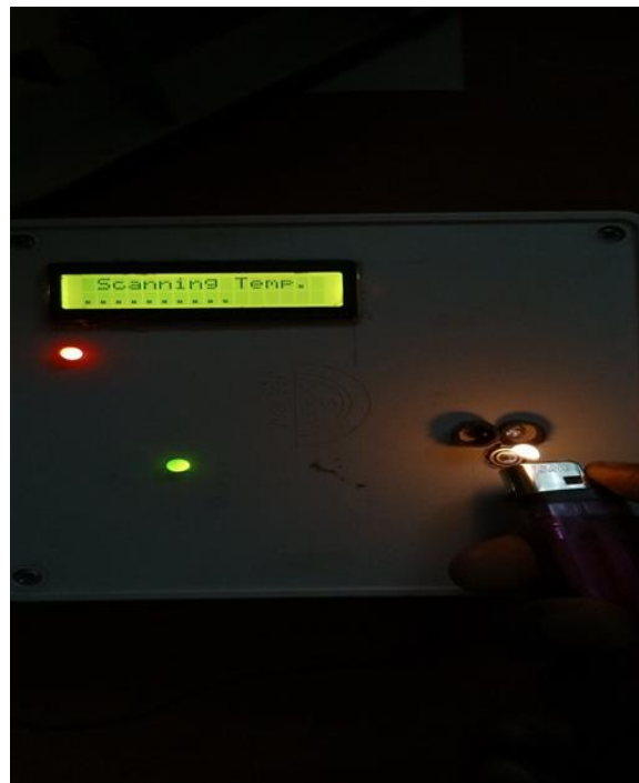
Fig.2. The process of heating the temperature sensor using heat/fire
