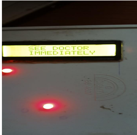
Fig.7. The system is instructing you to see a doctor because your temperature is above the expected or required temperature
