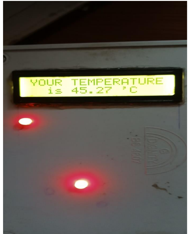
Fig.5. The system displays the amount of temperature it detects, which is above the required human temperature
