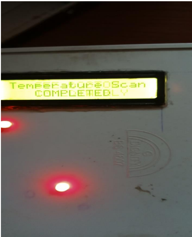
Fig. 3. The system has finished reading the temperature of the object/fire
