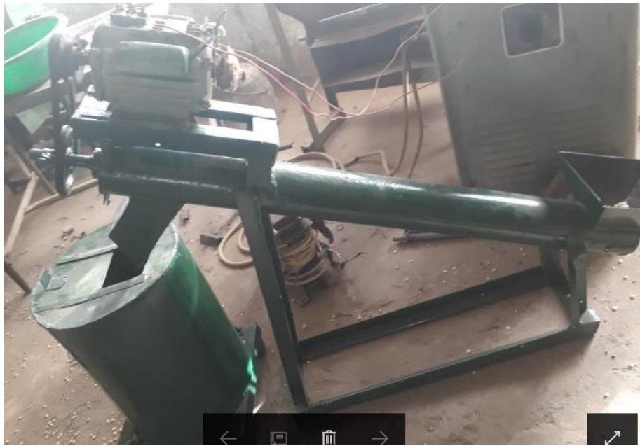
Plate-I: The developed conveyor and a metal silo of the post-harvest processing plant
