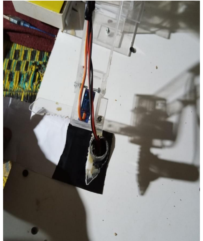
Fig.-10: Gripper opens at the picking point when it senses a black object.
