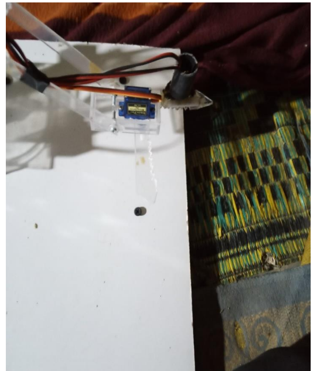
Fig.-12: The Gripper opens at the placing point to drop the black object it took from the picking point.
