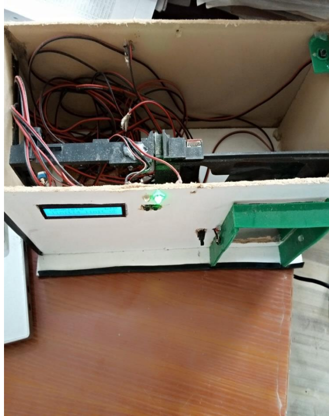
Fig. 4: Implementation of the Circuit Diagram of the Visitors Counter with Gate Control and Automatic Room Light Controller (ON/OFF)
