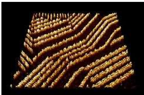
Fig.29: STM image of reconstruction on a clean gold (100) surface
